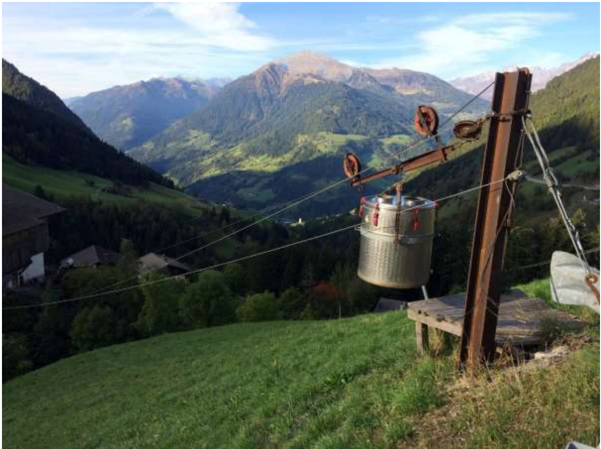
Figure 18. Zipline for milk transport in South Tyrol, Italian Alps (source: own photo, 2019).
