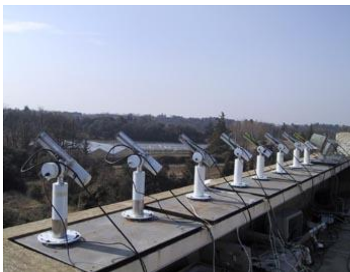
Fig 4.2. View of the instrument platform with eight sun-photometers in the Carpentras site (operated by MeteoFrance) used for outdoors radiometric calibration of other sun-photometers. Multiplied by 600 and covering the whole globe (or at least the continental surfaces of it), the networked sun-photometers interweave two twin narratives: instruments for producing scientific knowledge and troubling manifestations of Big Brother.
