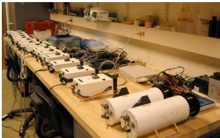
Fig. 4.3: Two SIMBAD (cilindrical) and several SIMBADA radiometers (tetraedrical), which measure the two basic parameters for the validation of ocean color: marine reflectance and aerosol optical depth.
