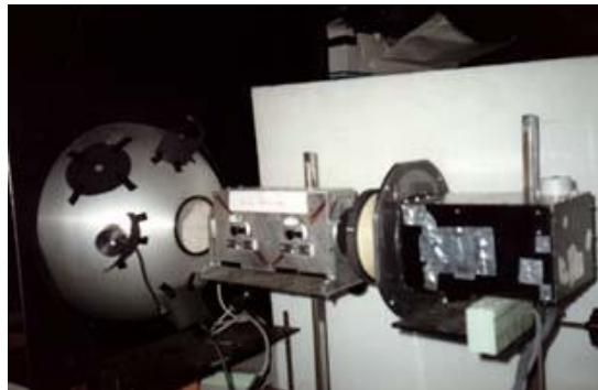
Fig. 2.3.: Calibrating the aircraft version of POLDER with the sphere. http://www-loa.univ-lille1.fr/Instruments/fr/polarimetres/polder/carac.php
