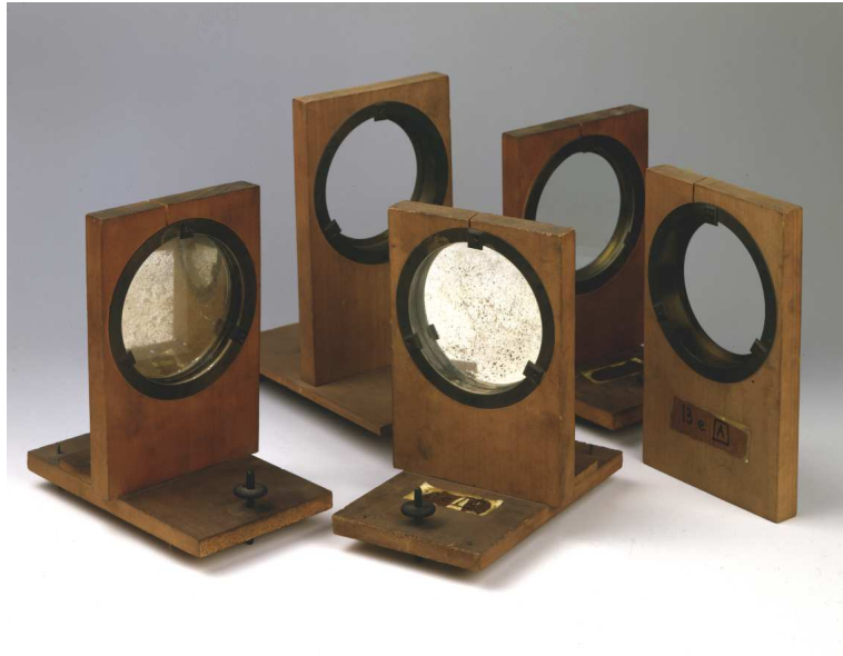
Figure 5. Mirrors and supports used by Léon Foucault for comparing the speed of light in water and air, 1862.
