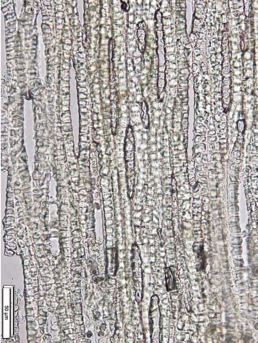
FIGURE 15 Sample No. 76 from Tsa Tsa Puri temple, room 3. Tangential section of poplar bark. The bark had remained attached to the roundwood sample. The rays are only visible as hollow shapes. The bark tissue is mainly composed of very long strands of chambered cristalliferous phloem parenchyma.
