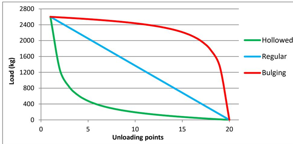
**Figure 4: Unloading patterns (example for 20 stops)**
