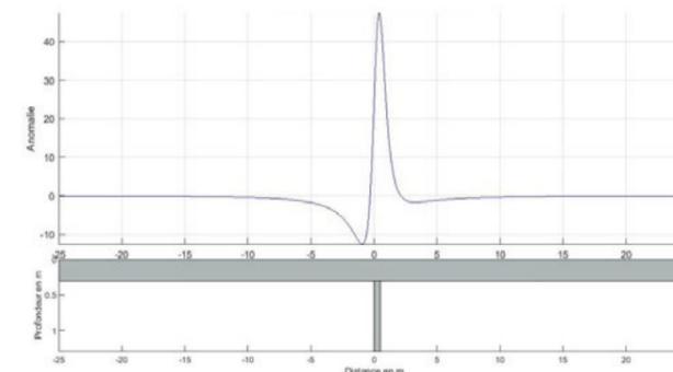
Figure 37: Magnetic anomaly caused by a “full” wall of 0.5 × 1 m at 0.3 m of depth (R. Al Khatib Alkontar, H. Reiller – MAFTOr/IPGS-EOST).
