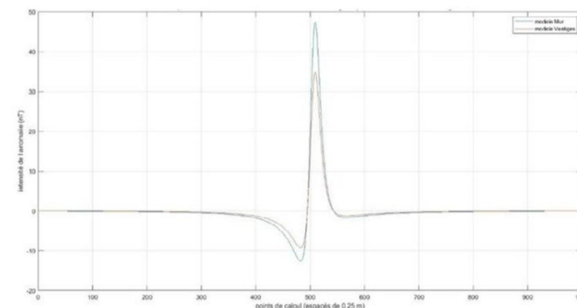
Figure 39: Comparison between magnetic anomalies caused by a “vestige” of wall (orange curve) and by a “full” wall (blue curve) (R. Al Khatib Alkontar, H. Reiller – MAFTOr/IPGS-EOST).
