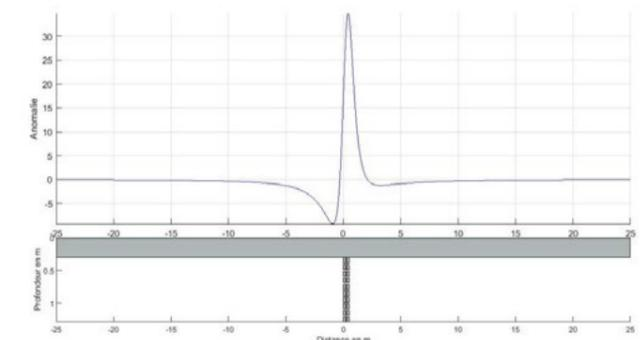
Figure 38: Magnetic anomaly caused by a “remain” of wall of 0.5 × 1 m at 0.3 m of depth (R. Al Khatib Alkontar, H. Reiller – MAFTOr/IPGS-EOST).
