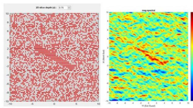
Figure 51: Magnetic anomaly caused by a wall of 1 × 1 m at 0.5 m of depth, surrounded by demolition rubble [75 %] (R. Al Khatib Alkontar, H. Reiller – MAFTOr/IPGS-EOST).
