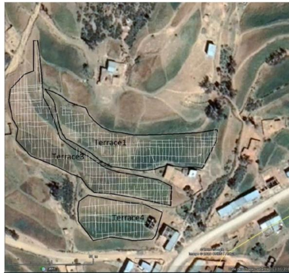
Figure 11: Profiles and tie-lines on terraces 1, 3, and 4 (R. Al Khatib Alkontar, H. Reiller – MAFTOr/IPGS-EOST).
