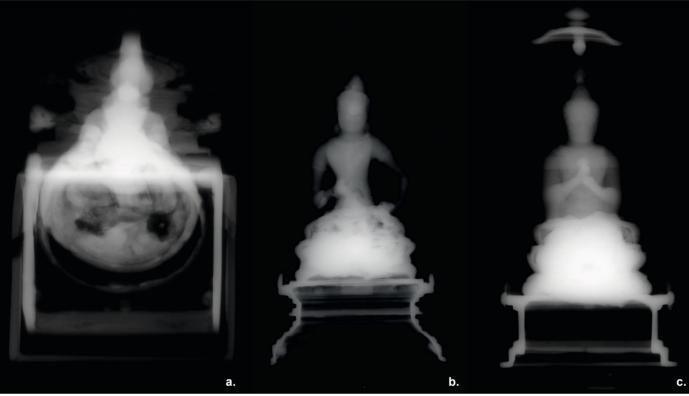
Fig. 45 — X-ray radiographs of MG 3625 (fig. 17) (a.), MG 2173 (fig. 14) (b.), and MG 18290 (fig. 15) (c.). The lead-tin material sealing the consecration deposits prevents the identification of the objects contained inside. Only for MG 3625 the white stone bead is visible (a black circle on the radiograph, see fig. 44a). Photo: © C2RMF/Elsa Lambert.
