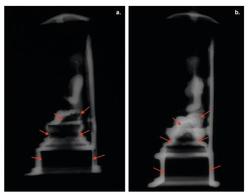
Fig. 26 — X-ray radiographs (left side view) of MA 5936 (fig. 10) (a.) and MG 2255 (fig. 9) (b.), showing the inner cavity in the pedestal, lotus and legs, as delimited by the red arrows. Photo: © C2RMF/Elsa Lambert.
