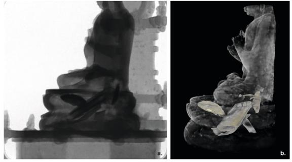
Fig. 46 — Neutron radiograph (a.) and tomography (b.) of MG 18290 (fig. 15) showing the objects of the consecration deposit inside the statue. Photo: © CEA-CNRS/Frédéric Ott (a.) & C2RMF/Elsa Lambert (b.).
