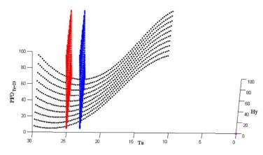
Figure 1: This picture represents the value of PPD as a function of Ta, for different values of Hy. Parameter Va is fixed to 0.2. The ten curves correspond to 10 fixed values of Hy from 0% to 100%. The red plane (resp. blue) cuts the PPD curves at value  $Ta = 25^{\circ}C$  (resp.  $Ta = 23^{\circ}C$ ). These planes clearly show that the value of Ta minimizing PPD depends on Hy. Source (Denguir, 2014, Fig 10).
