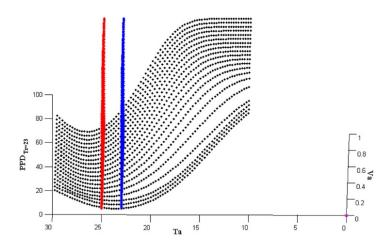
Figure 2: This picture presents PPD, as in Fig 1. More specifically, Hy is now fixed to 50%, the ten curves represent PPD as a function of Ta, for ten values of Va from 0 to 1. Source (Denguir, 2014, Fig 11).
