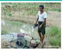
Engine pump used for irrigation.
