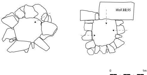
Fig. 7d: cesspit in the courtyard of a house (left); cesspit 33,94 in the street C4 North (right) the arrows indicate the probable income of the sewage
