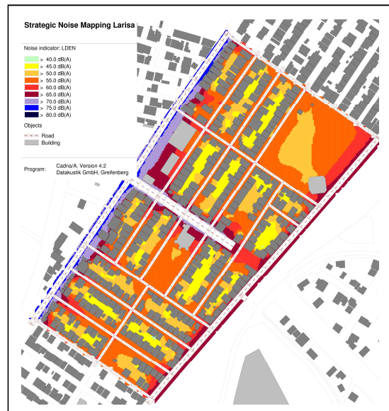
Figure 4: SNM: Lden simulation (Larissa SNM- Greece - UA of Echekratida): visualization of silence islet in between buildings blocks
