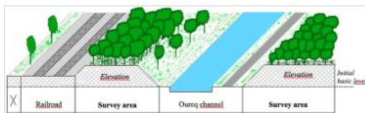
Figure 5 : Drawing showing the two infrastructures, the channel below the rail tracks and the artificial berms
