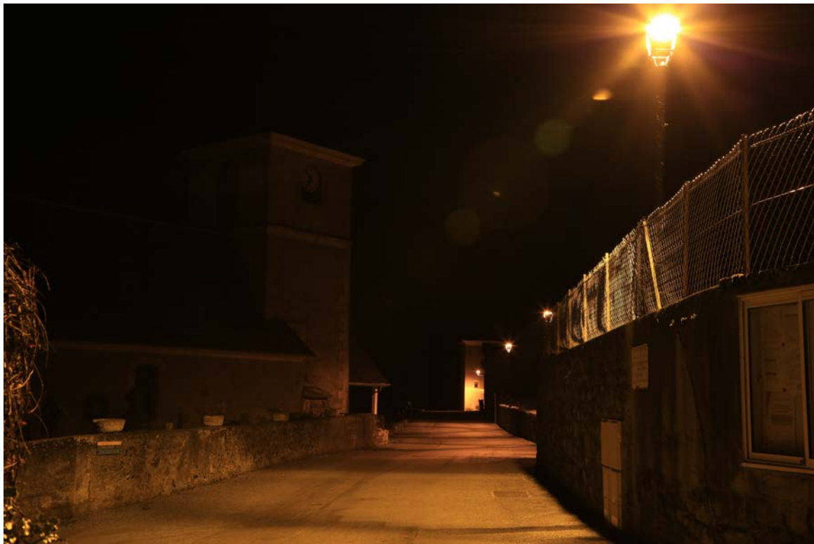
Main street of Ouzous. Full cut off lights; high pressure sodium lamps; 2200 °K; 8 lux.
