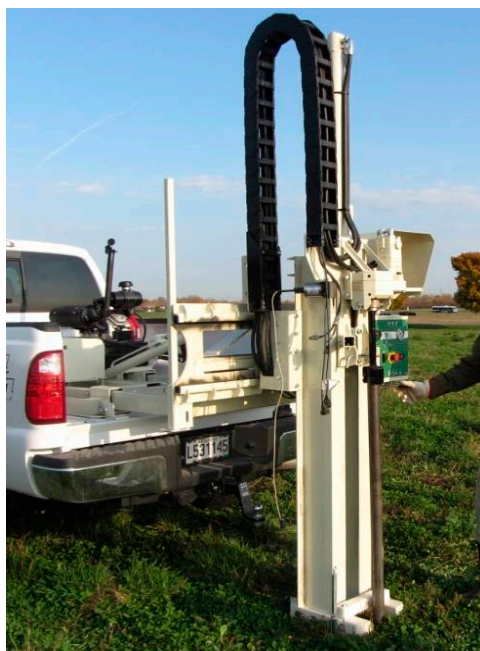
Figure 5. Veris ® P4000 unit with hyperspectral, EC_a and force sensors.
