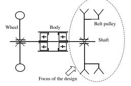
Figure 1. The schema of the product to design
