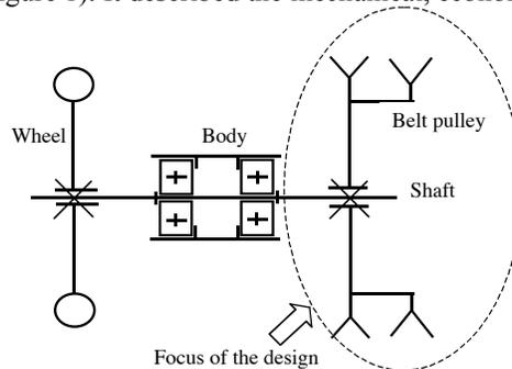
Figure 1. The schema of the product to design
