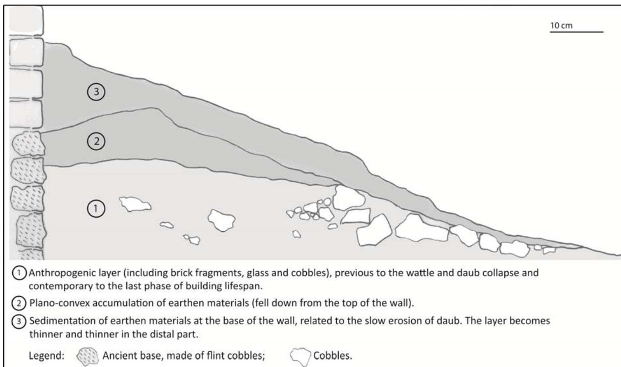
**Fig. 22.4** Cross section of a layer resulting from the sedimentation of earthen materials at the base of a wall (Cf. Fig. 22.5b, c ) in Rambures (Somme)
