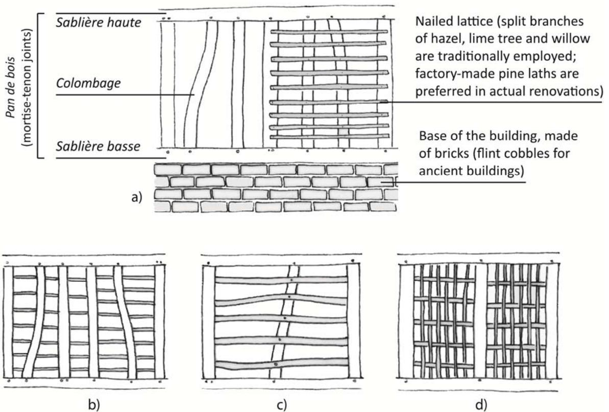
**Fig. 22.1** Examples of variability in timber frameworks from Northern France: ( a ) few spaced to moderately spaced laths, recorded in the Departments of Somme, Oise, and Pas-de-Calais; ( b ) *barreaudage* (horizontal bars) fixed by notches on the timber framework, recorded in Haute Normandie and in western Oise; ( c ) *gaulettes* (thick and spaced bars), recorded in Normandie (Marais Vernier); ( d ) Flemish vertical wattle, that can be horizontal in some areas of Pas-de-Calais.
