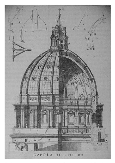
$\textbf{Fig. 1} \quad \text{Elevation and section of the damaged cupola of St Peter's, juxtaposed with force diagrams} \\ \text{(From Jacquier et al. [1742])}$
