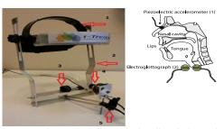
Fig. 1: (a) Multi-sensor Hyper-Helmet: 1) Adjustable headband, 2) Probe height adjustment strut, 3) Adjustable US probe platform, 4) Lip camera with proximity and orientation
