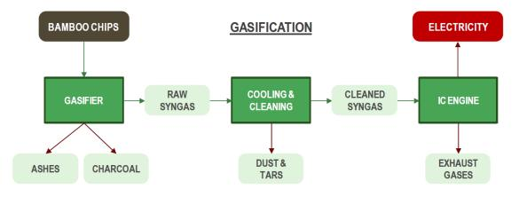
Figure 5. Gasification general process flow(Kerlero de Rosbo and de Bussy, 2012)
