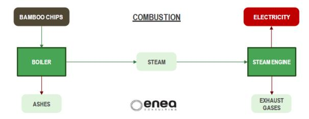
Figure 3. A diagram of combustion process from bamboo biomass to electricty(Kerlero de Rosbo and de Bussy, 2012)
