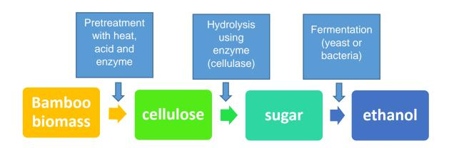
Figure 7. Simplified process of producing ethanol from bamboo biomass
