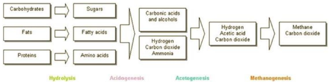
Figure 6. Anaerobic digestion pathway (Girard, 2013)
