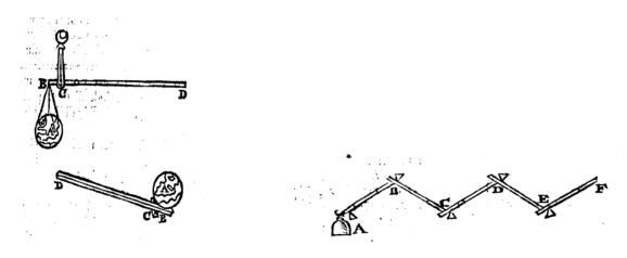
FIGURE 1: Wilkins' illustrations of Archimedes' idea to lift the earth and of the multiplication of force by the combination of levers (p. 81 and 84).
