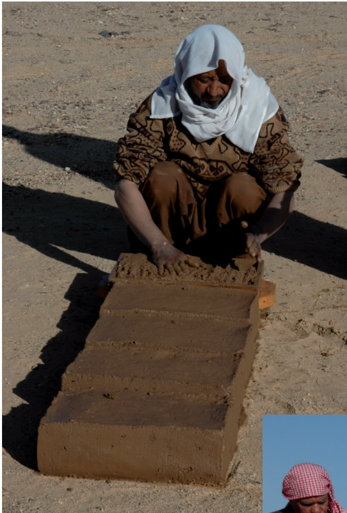
Fig. 9. Mudbricks left to dry
