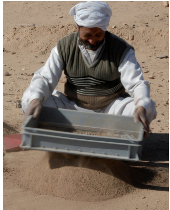
Fig. 2. Loam crushed and being sieved with a 4 mm sieve
