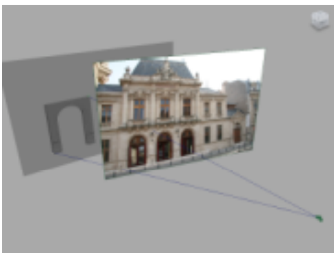
Figure 4: Using a photograph for the 3D reconstruction process: positioning 3D point in the scene with the help of a viewpoint recovery picture and a positioned plane.
