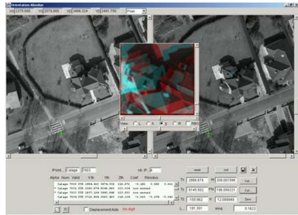
Figure 3. Stereo-window in the middle of the screen (anaglyph technique), as an example in the window of absolute orientation.
