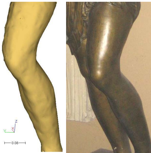
Figure 10. Model after smoothing the mesh (left) compared to the original image (right).
