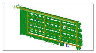
Figure 4. Detection of only two planes when data are segmented using t = 350 mm.
