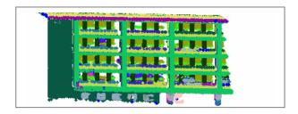
Figure 5. Successful segmentation with t = 40 mm.
