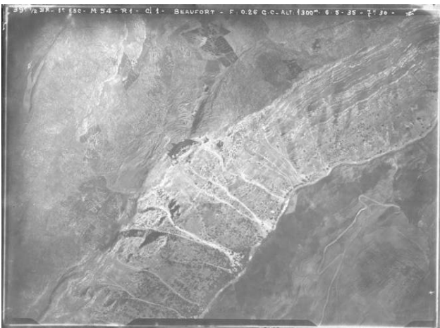
Figure 4. Example of archive photo of 1935 (DGA, area of Beaufort's castle), showing the castle (in the middle) and the landscape (focal length 26cm, flying height 1300m above ground, 2000m above sea level)
