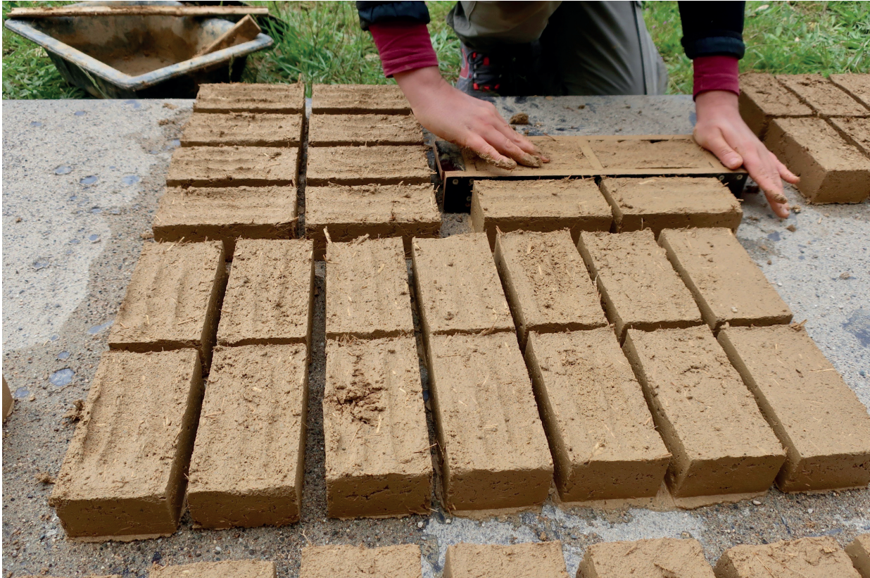
Figure 4. Moulding small mud-bricks. © María Lidón de Miguel.
