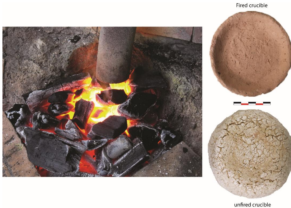
Figure 4: On the left, the smelting hearth with the bent tuyère above the charcoal-covered crucible. Bottom right, exterior of the unfired experimental crucibles and top right, interior of the fired experimental crucibles
