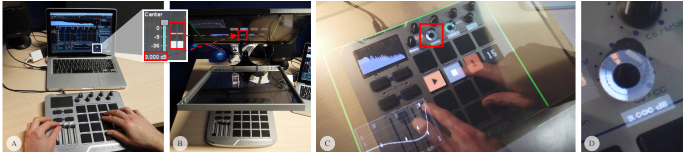
Figure 1. ControllAR enables the appropriation of visual feedback on control surfaces. Elements from the GUIs of controlled applications (A) can be cut, transformed and rearranged (B) by users. They can then be placed on/around sensors on the controller using an optical combiner (C). Close-ups show the value of the volume parameter of a track and the resulting VU meter being placed around the knob that controls it (D), illustrating both process and parameter feedback.
