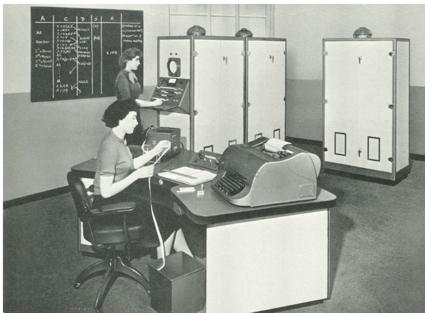
Figure 3: The STANTEC ZEBRA computer. The blackboard displays a typical example of Van der Poel’s programming style with arrows indicating the timing relationships between the instructions.
