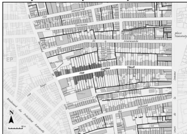
Figure 6 - Land parcel limits of the cadaster of 1851 (in black) copied on the current cadastral plan: one after the other, each owner has subdivided its parcel. (Drawing of Ch. Callais according to cadasters)
