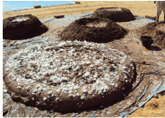
Fig. 13.9 Temper spread on top of trampled mound
