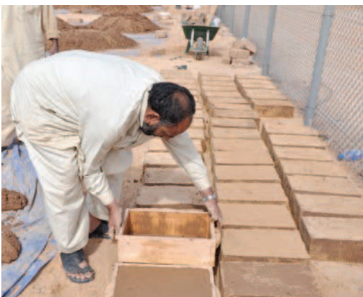
Fig. 13.16 Removal from the mould
