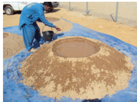
Fig. 13.5 Pyramid-shaped mound with central crater filled with water
