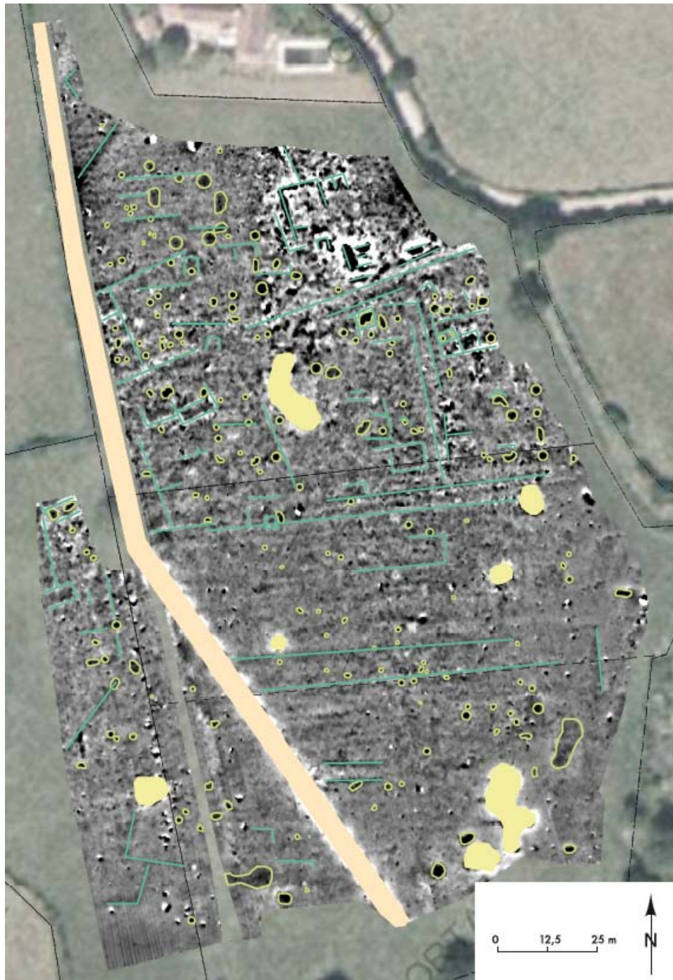
Magnetic prospection (scale =-4 to 4 nT/m) : orthography (Géoportail), administrative limits and anomalies
