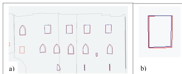
Figure 4. Surveying measurements (connected in blue) and point cloud digitizing (red); a) Eastern facade; b) Zoom on a rectangular reveal window.
