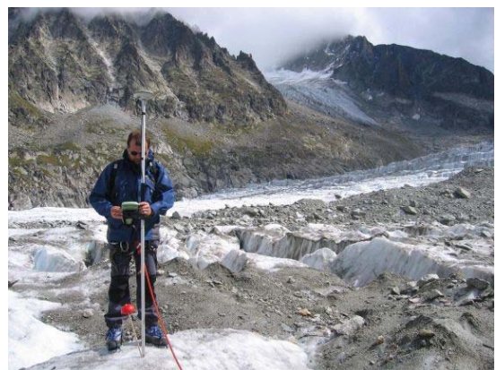
Figure 4. Rapid static GPS measurements (Mer de Glace)
