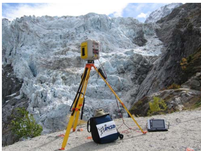
Figure 7. Laser Scanning of the glacier front
