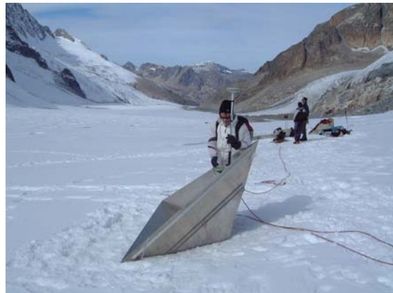
Figure 3 : Measurement of the position of a corner reflector by GPS (Argentière glacier).
