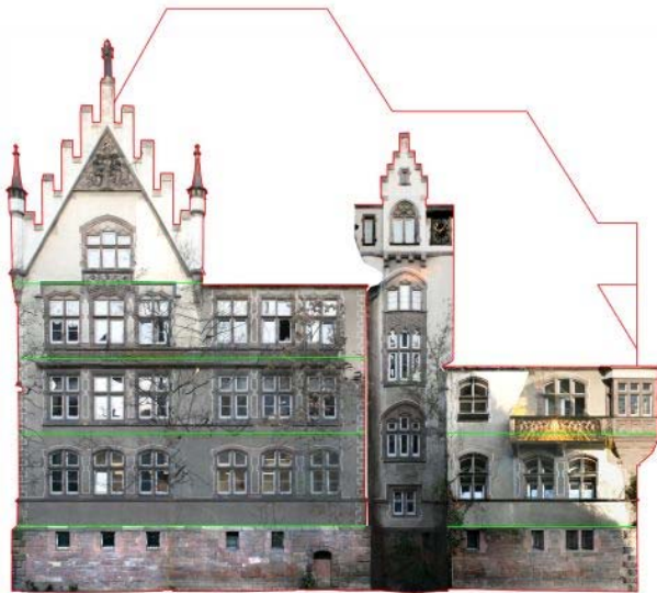
Fig. 4. Example of orthophoto (Building C) imported into AutoCAD® software and used as reference documentation for all providers.
