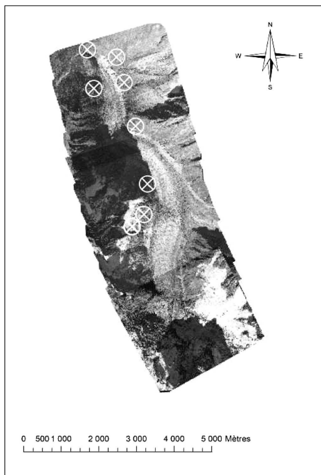
Fig. 3. Layout of the set of 13 photos that were taken over the Mer de Glace in 1995 and are entering in the AT processing. Circles represent the points measured by GPS.
