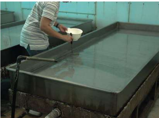
PHOTO 19 Removing fine precipitated floating matters with a scoop.
