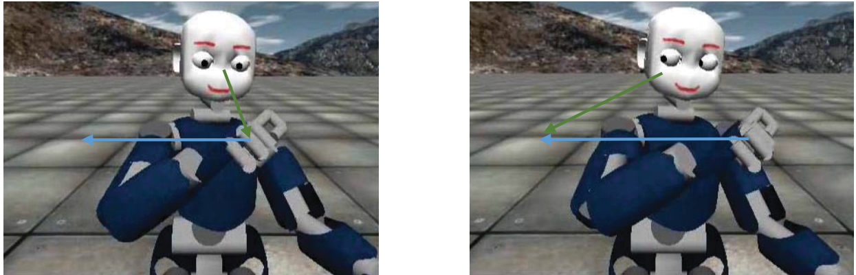
Fig 1. The simulated iCub robot. The robot is acting as the leader in the mirror game, generating random sinusoidal trajectories. (Left) the gaze is fixated on the hand. (Right) the gaze precede the hand. The blue arrows shows the next hand movement and the green arrows show the current gaze fixation point.
